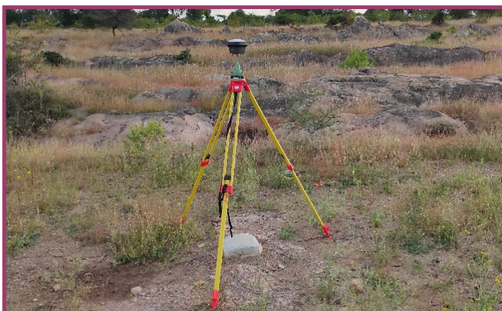
[Borehole survey works using DGPS instrument at Neerbudhihal Limestone Block, Bagalkote (Dist.)]
